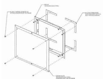
Place a load spreader at each corner and fix with the supplied scews.
